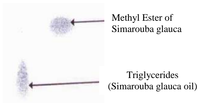
Figure-2 Thin Layer Chromatographic analysis. Triglycerides (Simarouba glauca oil) and Methyl Esters of Simarouba glauca
