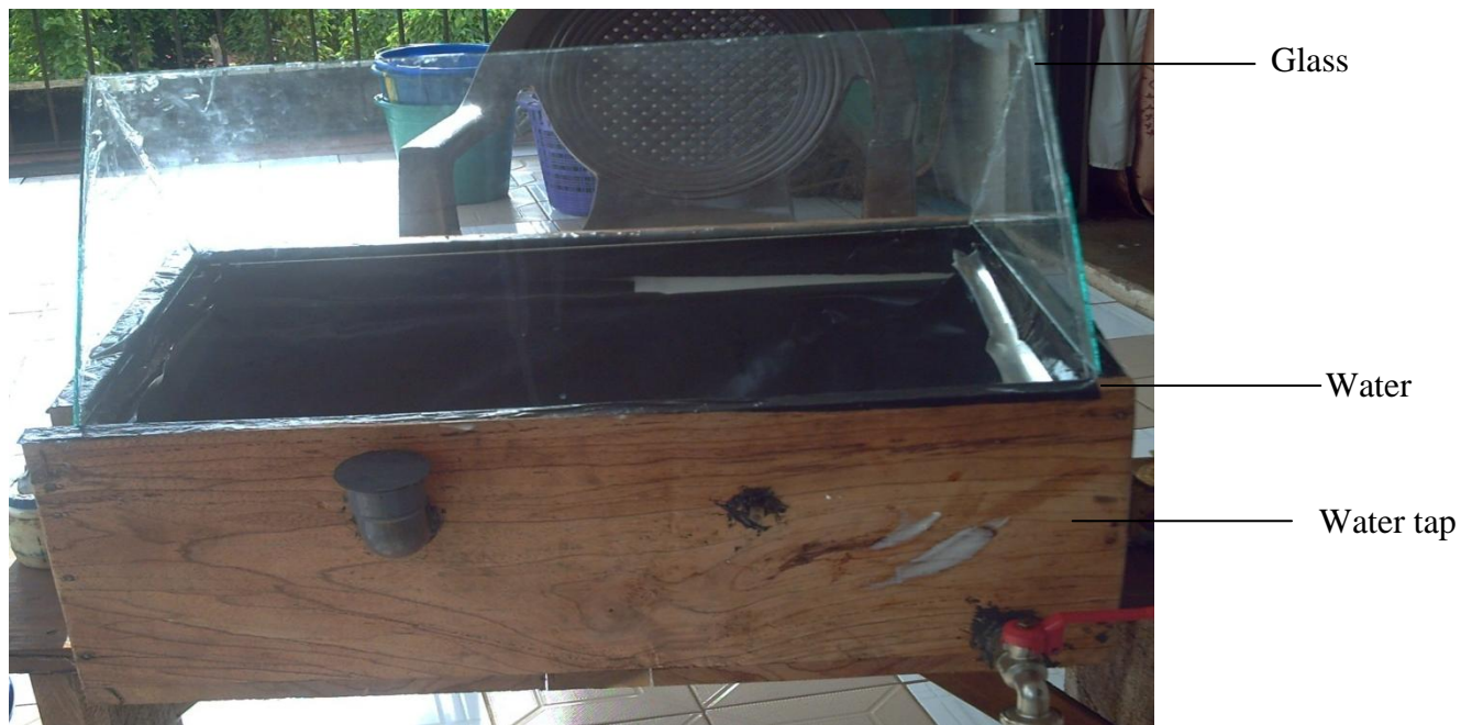
Figure-2 The glass roof on top of the rectangular water tank
