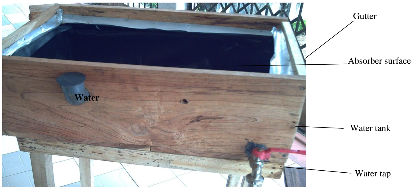
Figure-1 The rectangular water tank on top of RSWD stand
