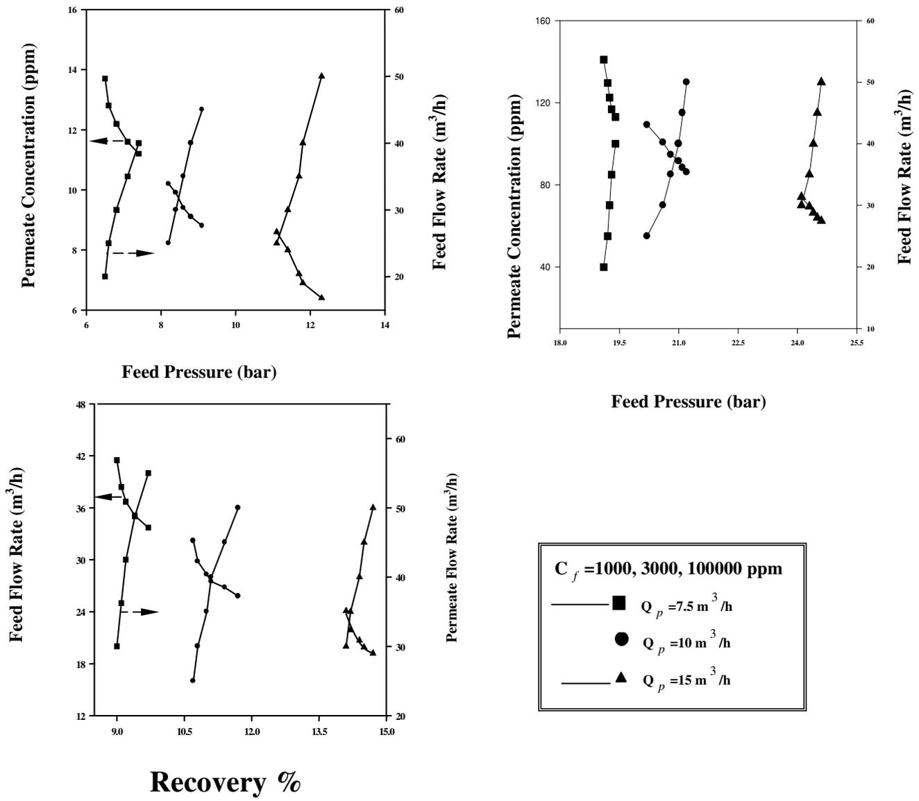
Figures-5, 6 and 7: show the Influence of feed pressure and feed flow rate on the optimum concentration of permeate water with various feed water concentration.
