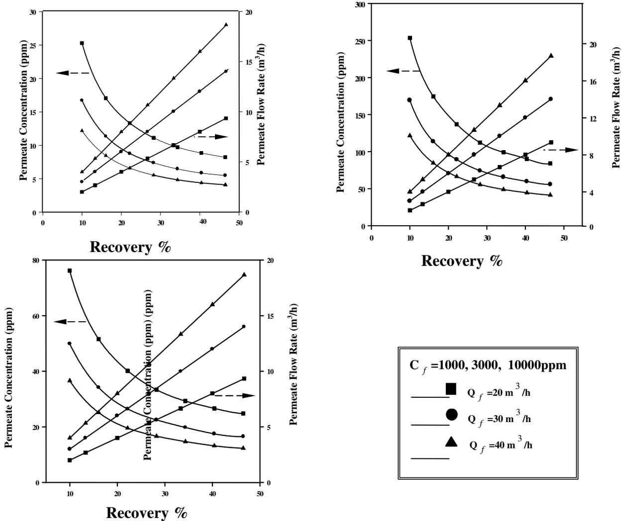
Figures-1,2 and 3: show the Influence of percent recovery and permeate flow rate on the optimum concentration of permeate water For different feed water concentration
