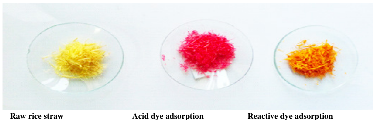
Figure-5 Schematic prototype of adsorption of acid and reactive dye on the modified rice straw
