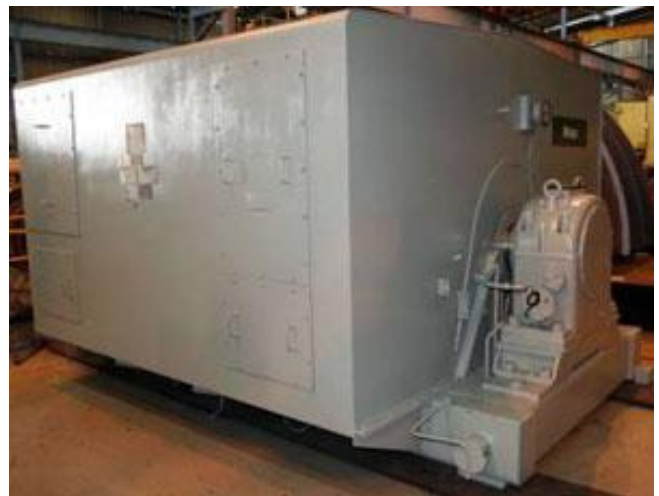
Figure-1 Image of 13.7 Mw High voltage Induction motor
